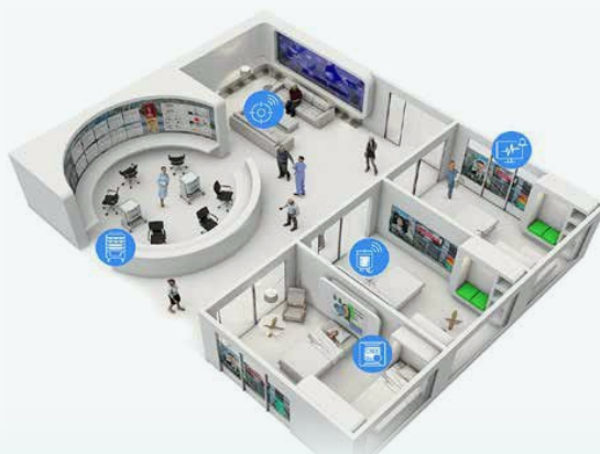
Smart patient ward: nurse call, IPTV, monitoring and building control on one network
